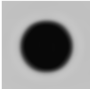
(a) 100 kV at 650 \mu\text{A} , 0.4 mm focal spot.
